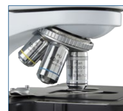
● S100x oil objective with built-in iris diaphragm
