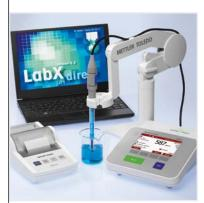
Upon endpointing SevenCompact™ allows multiple archiving options: the data can be stored, printed or transferred to EasyDirect pH. Any combination of these three options is possible giving you total flexibility.
