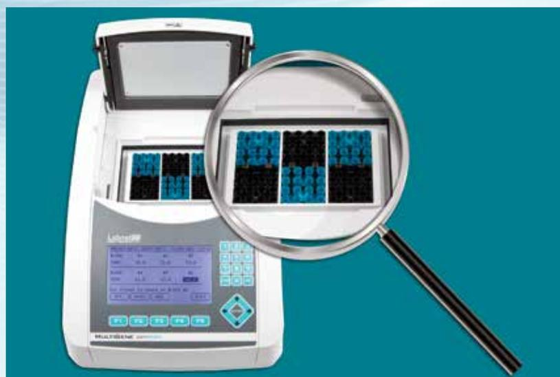
The 6 distinctive blue and black peltier elements on the 96 well block can each be set to a unique and distinctive annealing temperature in your single method.
