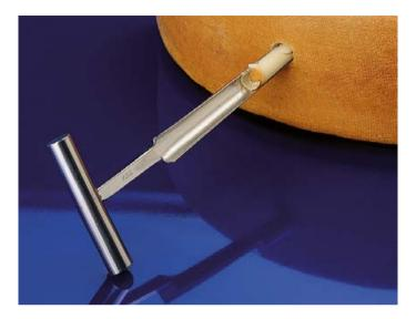
Conical hand-drill, conically shaped, with sharp cutting edges and a solid handle. Ideal for cutting out samples for quality control from soft, paste-like substances (cheese, butter, clay, soap, wax, etc.).
