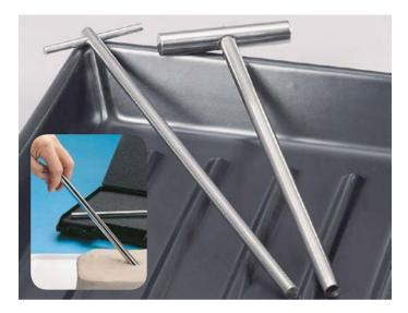
Cylindrical hollow drill with a sharp cutting edge, can easily be driven into paste-like and semi-solid substances. The samples cut out are subsequently removed with the appropriate push-rod ejector. Total length 260 mm. Inner  $\emptyset$  8 mm, outer  $\emptyset$  10 mm.
