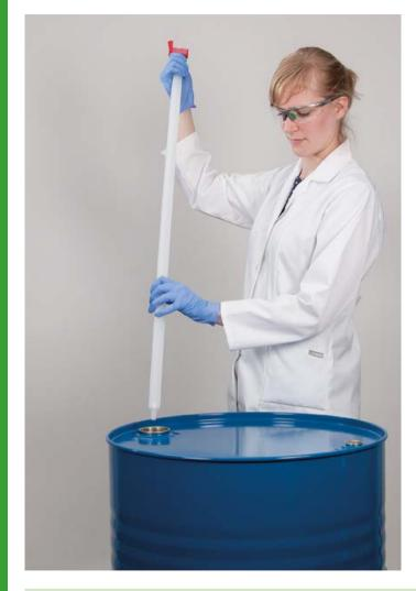
Dip sampler for simple removal of liquid samples. Good view due to transparent tubes. Upper end with reflux valve, lower end with ball valve.
