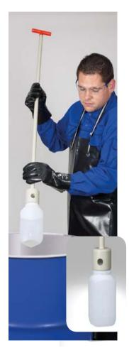
The ChemoSampler was developed for sampling aggressive liquids, e.g. acids, alkalis, detergents. The samples are drawn directly into the screw-on original sampling bottle. The tamperproof bottle closure of these bottles with original safety ring ensures unadulterated sample transport. Samples can be taken from depths of as much as 200 cm, e.g. from tanks, silos or tankers, by using the extension rod.
