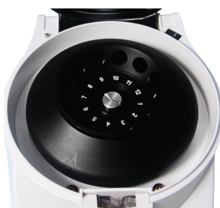
Fixed angle rotor (included) for 12x 0.2/0.5/1.5/2.0ml tubes
