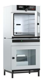
The direct contact between the load and the heatable and removable thermoshelves in the chamber of the Memmert vacuum oven VO ensures rapid and uniform temperature control of food, cosmetics, watches, books, PCBs or injection moulds, without the loss of heat.
