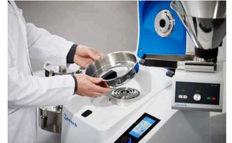
A push-fit system without screws and the patented cassette principle allow for easy insertion and removal without tools.
