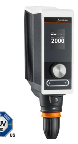
The Hei-TORQUE Expert 100 is a overhead stirrer with a wide speed range (10 - 2,000 rpm) and a maximum torque of 100 Ncm. With it you can optimally stir viscosities up to 60,000 mPas or volumes up to 50 liters ( $H_2O$ ).
