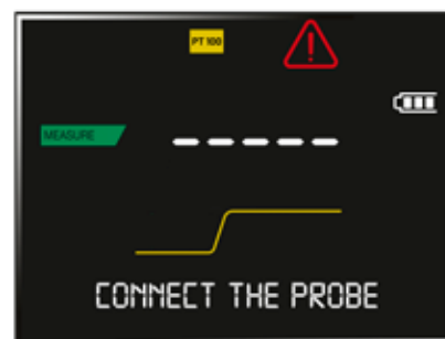
Color backlit LCD display with self-diagnosis messages
