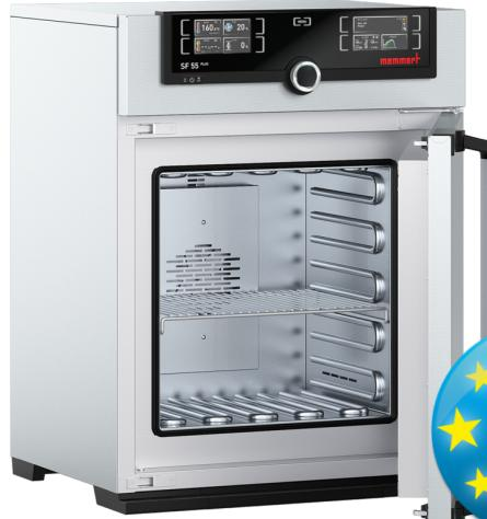
The indispensable safety feature for this hot air steriliser: Setpoint Wait. This means that the programme for sterilisation only starts when the set temperature has been reached. This feature can also be used with freely positionable Pt100 temperature sensors. Here the sterilisation time only begins when the set temperature has been reached at all measurement points, and reliable sterilisation is guaranteed at all times.
