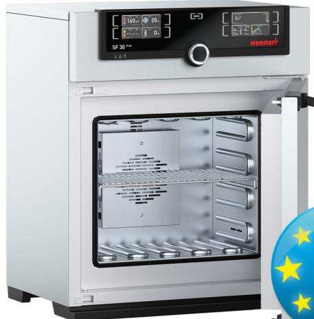
The indispensable safety feature for this hot air steriliser: Setpoint Wait. This means that the programme for sterilisation only starts when the set temperature has been reached. This feature can also be used with freely positionable Pt100 temperature sensors. Here the sterilisation time only begins when the set temperature has been reached at all measurement points, and reliable sterilisation is guaranteed at all times.
