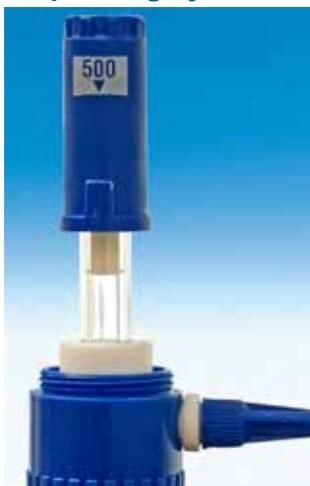
The direct displacement system of the **MINISPENSOR** is for universal use and ideal for crystalline solutions.
