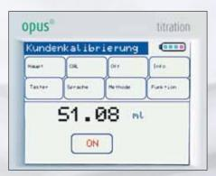
The Quick-Cal configuration menu enables individual calibration, easily and reliably.
